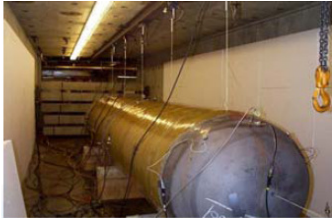
Figure 11: CNG steel container (courtesy of TransCanada)
