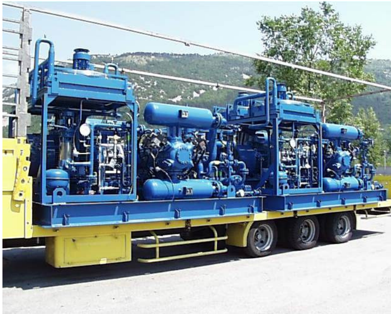
Figure 7: Evacuation compressor unit on a truck (courtesy of HGC, Hamburg)
